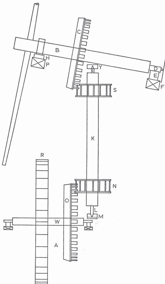
Fig. 21. The machinery of a drainage mill (simplified)
