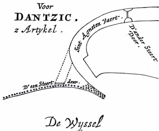
It is obvious that there is great depth in front of the wooden dam of the St. Agnes Channel, as much (so they say) as four or five fathoms, but behind the pier there built in the channel, sand accumulates according to the general nature of such piers; therefore the channel should be dammed at that pier and excavated to a great depth, as the annexed Figure shows:
