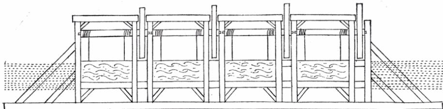
In the Mottlau near the Theerhof three or four vertical gates should be built, side by side, which may have the shape shown in the annexed figure; and an equal number of doors in the Mottlau near the Langgarter Thor.
